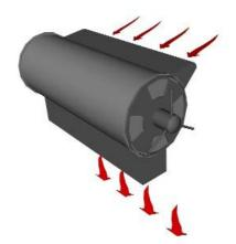
DRYING SYSTEM - Our Unique highly efficient drying system uses 100% of the tightly controlled process air through the product bed itself for unbeatable performance. Outlet air exhaust slot is placed in the opponent side avoid any kind of air turbulence in the spray zone. To further enhance process efficiency, Drying flow direction is automatically inclined to the core's bed according to the batch quantity, shape of product or phase of the process. Easy to be cleaned and dismantled.
