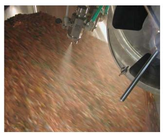
Powder Dosing System Automatic powder dosing is available very versatile and with high accuracy. A new patent system avoids any powder clogging while dosing.
