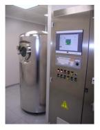
**MICROLAC CONTROL SYSTEM** – A very sophisticated but user **friendly** software has been designed by Nicomac. PLC based control system guarantees complete automatic process repeatability. HMI (human machine interface) with touch screen industrial PC for flawless data acquisition and storage. The Microlac software stores up to 40 different recipes with up to 99 discrete phases.
