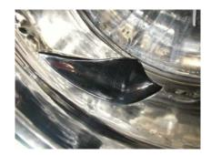
**SOLID WALL COATING PANS -** Our coating systems utilize a smooth, electro-polished, non-perforated, solid wall pan. The solid wall design combined with our unique drying system has unsurpassed coating performance. In addition, solid walls make for a more thorough and easier to validate cleaning process.
