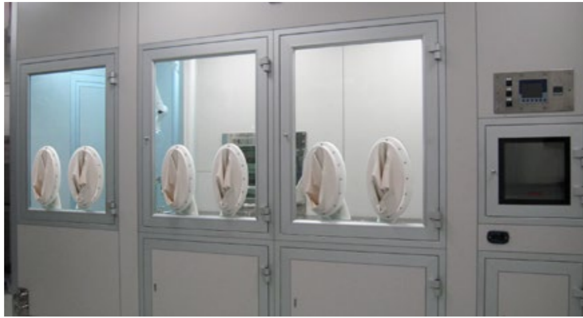
RABS (Restricted Access Barrier System) with Nicomac walls and pass box
